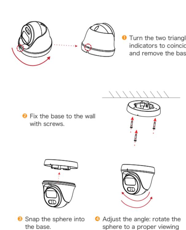
1 Turn the two triangle indicators to coincide and remove the base.
