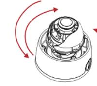
1 Loosen 4 screws and remove the cover.
