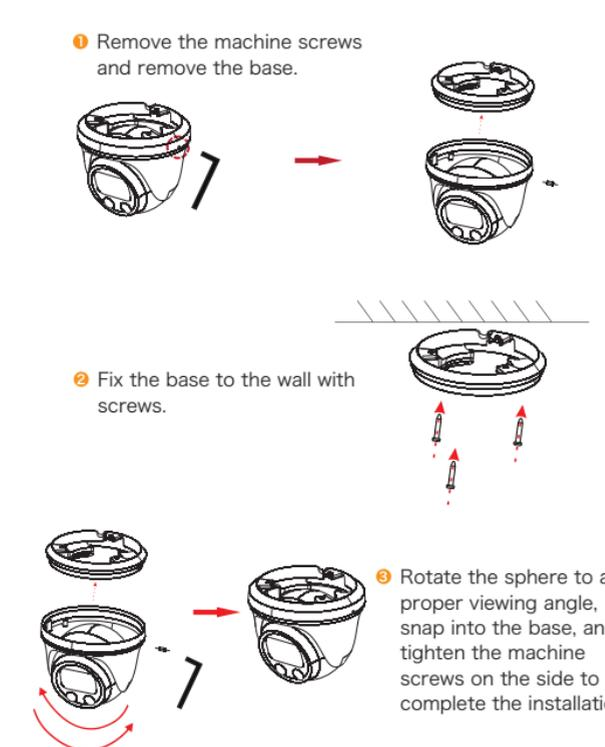
1 Remove the machine screws and remove the base.
