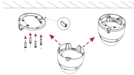
1 Remove the rubber plug and fix the base with 4 screws.
