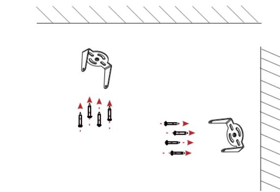
2 Use 4 screws to fix the bracket to the ceiling or fix it to the side wall.
