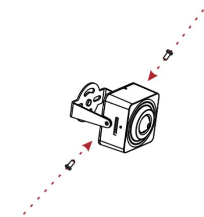
3 Adjust the viewing angle, tighten the screws, and complete the installation.
