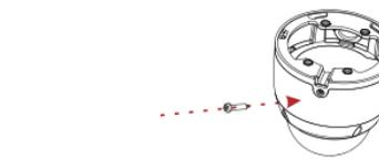
3 Lock the screws, fix the ball, and complete the installation.
