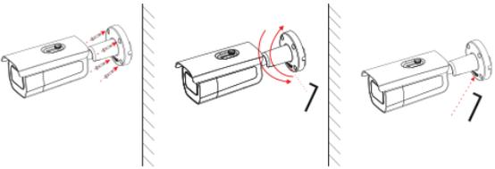
1 Fix the bracket to the wall with screws.
