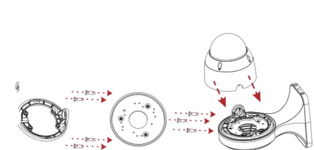
1 Fix the base and bracket mounting plate to the bracket body with screws.
