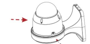
3 Fix the camera screw and complete the installation.
