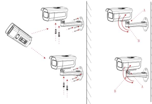
1 Fix the camera to the bracket with screws. The bracket head can be pre-mounted or post-mounted, and then fixed to the wall with screws.
